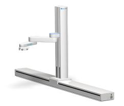
With the vertical column work envelope and embedded controls, PreciseFlex sample handlers offer the highest workspace density, saving valuable floorspace.
