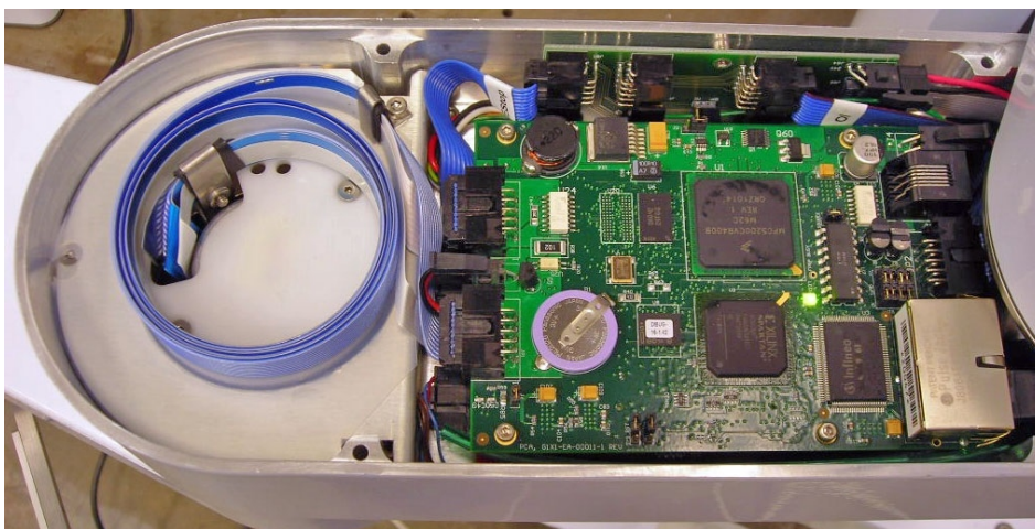
Figure 2-2: Controller Installed in Inner Link
