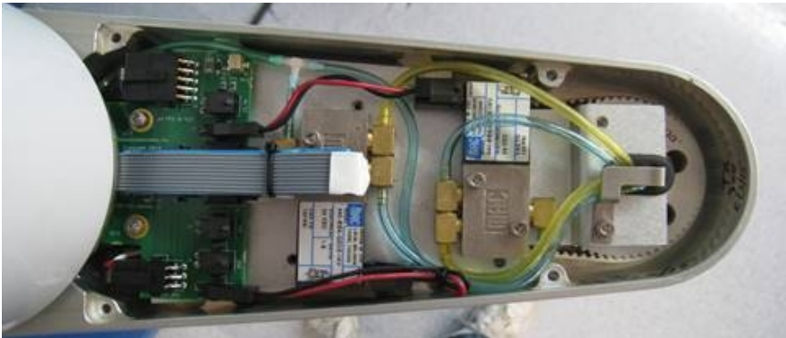
Figure 2-12: Dual Pneumatic Gripper Configuration (with Rev C Sheet Metal, 2016)
