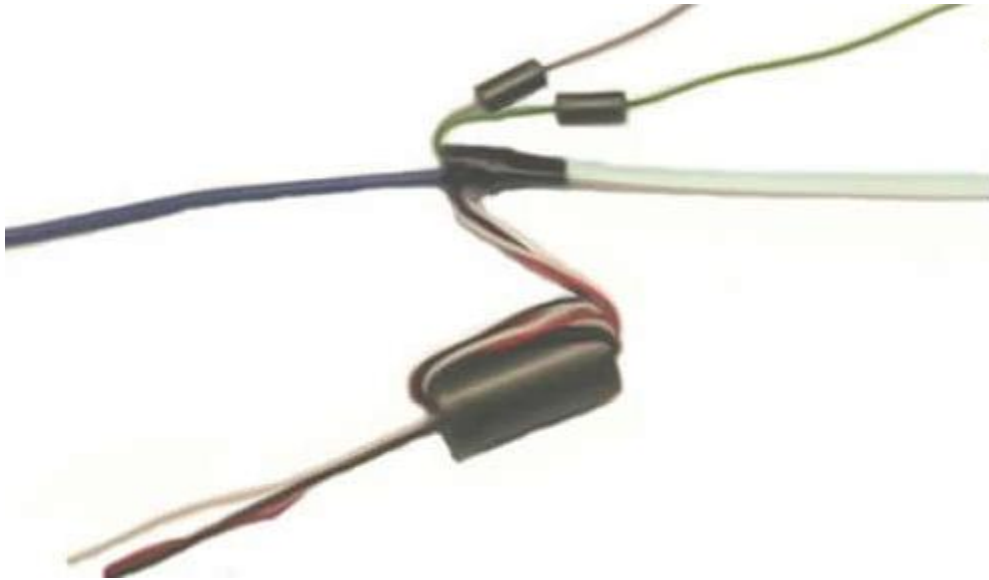
Step 3: Three motor wires looped three times through large core
