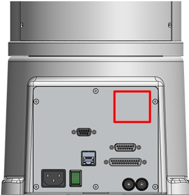
Location of the Product Label on the Facilities Panel at the Base of the Robot
