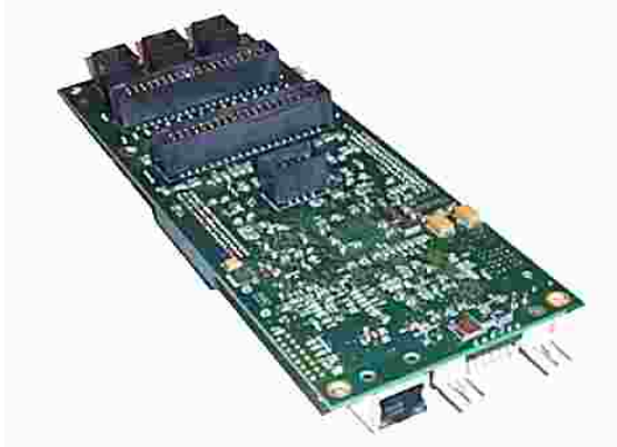
Figure 2-5: Enhanced RIO Module
