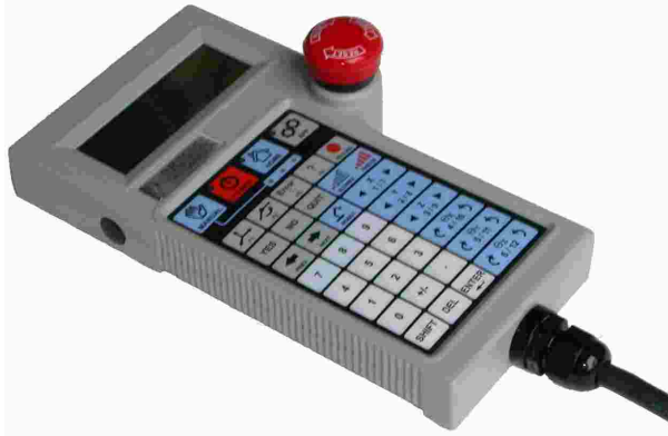
Figure 2-4: Manual Control Pendant
