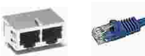
Figure 4-14: Ethernet Ports and Cable
